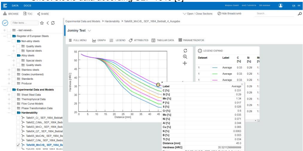
Figure 6: Parametrized Jominy model for hardenability with different levels of Cr
